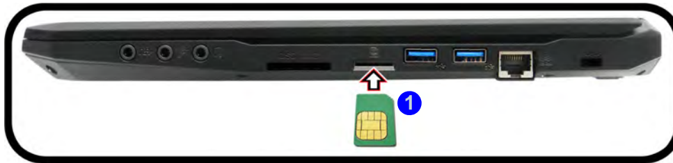
Figure 1 - 10 USIM Card Insertion
